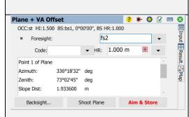
In a conventional survey, use the Measure points on a plane measurement method to define a plane and then measure points relative to the plane.
